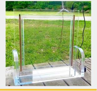
Power generation from both sides and all edges when photons reach the photovoltaic layer
